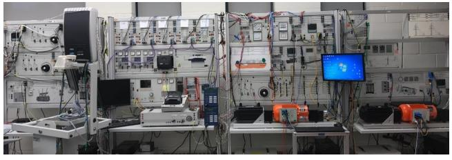
Fig. 4. The functional microgrid at SUNY Buffalo State Smart Grid Lab
