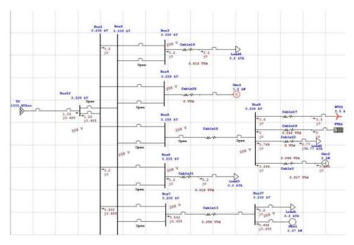
Fig. 1. ETAP® Load Flow study of proposed configuration
